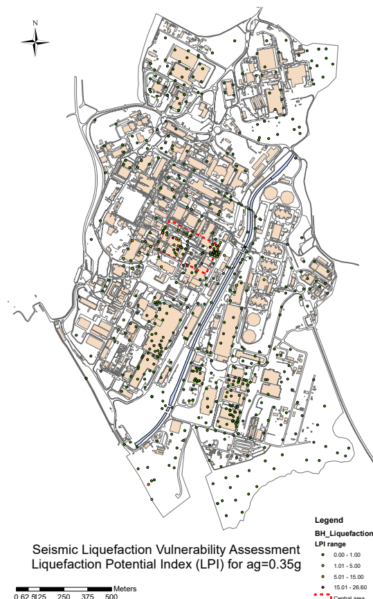
Figure 5: Distribution of the Liquefaction Potential Index at Sellafield for 0.35g peak ground acceleration
