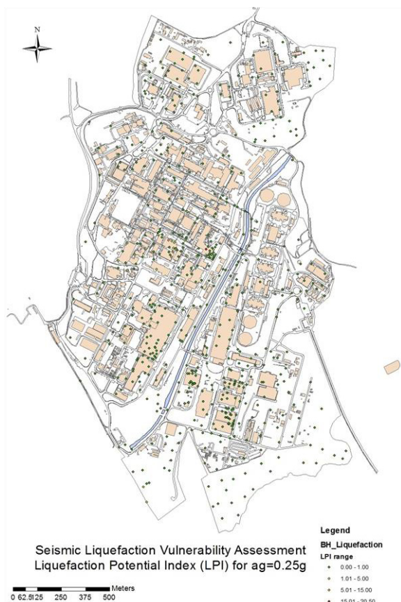
Figure 3: Distribution of the Liquefaction Potential Index at Sellafield for 0.25g peak ground acceleration
