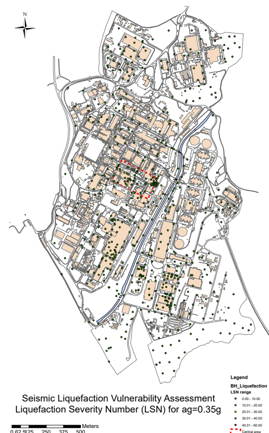
Figure 6: Distribution of the Liquefaction Severity Number at Sellafield for 0.35g peak ground acceleration
